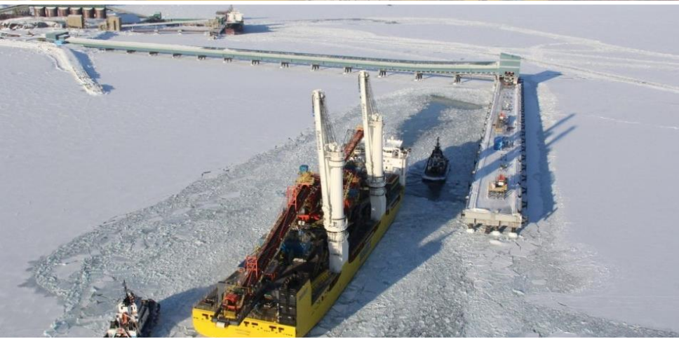
SHIPLoader IN HIGH WATER LEVEL POSITION: (BOOM AT +16° - MEASURED FROM THE COUNTERWEIGHT)
